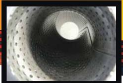
Perforated tube high flow muffler internals supported with a case stiffener.
