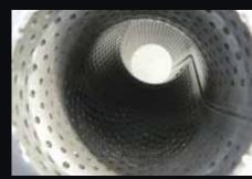
Perforated tube high flow muffler internals supported with a case stiffener.
