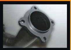
I 0mm thick 4 bolt pipe through flange design for perfect fitment accuracy.
