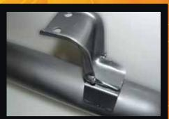
O.E. style heavy duty hangers and brackets connect to all orginal mounting points on vehicle.
