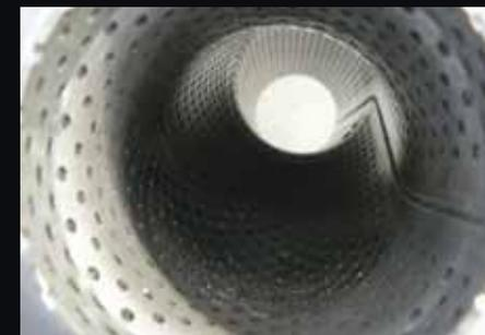
Perforated tube high flow muffler
